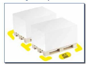
In factories and warehouses, a common floor marking scenario involves marking a series of boxes on the floor. Whether the objective is to create a pallet alignment system or a work cell, the basic layout is the same. An easy way to mark a series of boxes is with a combination of X-markers, T-markers, and corner markers. Corner markers mark the outside edges of the box, and T's and X's are used to divide the inner edges of adjacent boxes.
